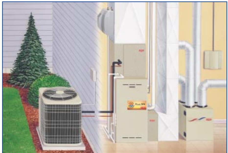
Central Air Conditioner and Gas Furnace System
