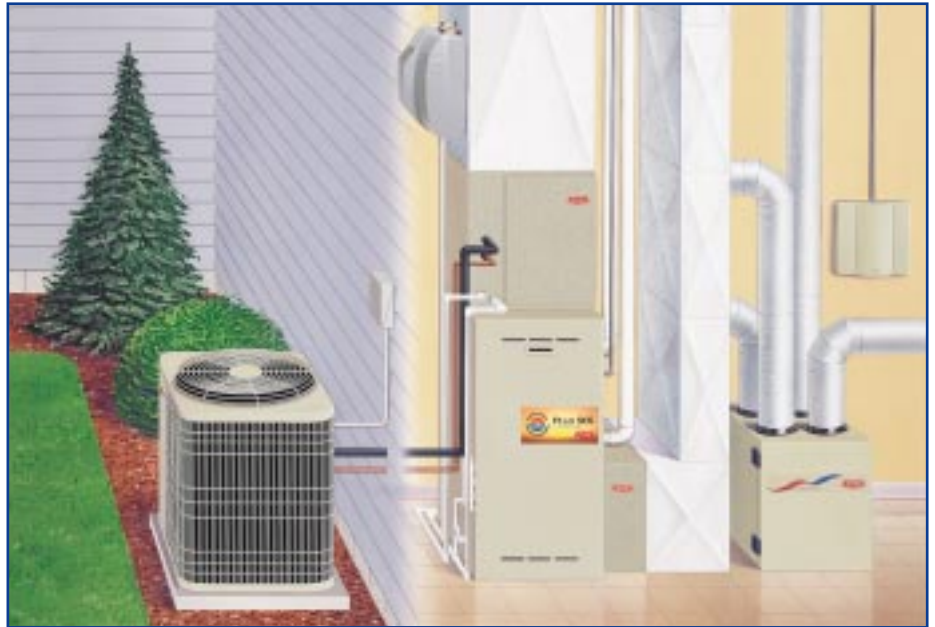
Central Air Conditioner and Gas Furnace System
